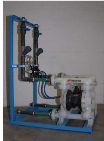
Dual 1 1/2" Air Diaphragm pumps
