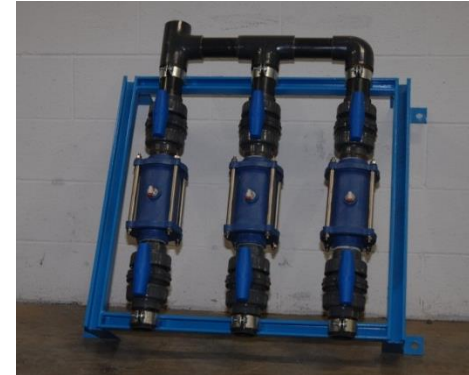
1 1/2" Pinch Valve Rack
